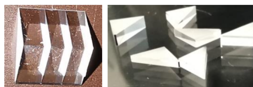
Figure 4. Optical microscope images of cutting 3.0mm thick glass prism by AOC ps-1064nm laser
