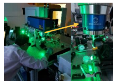
Fig.2 Arges Multi-axis precision drilling head with fs-515nm laser.
